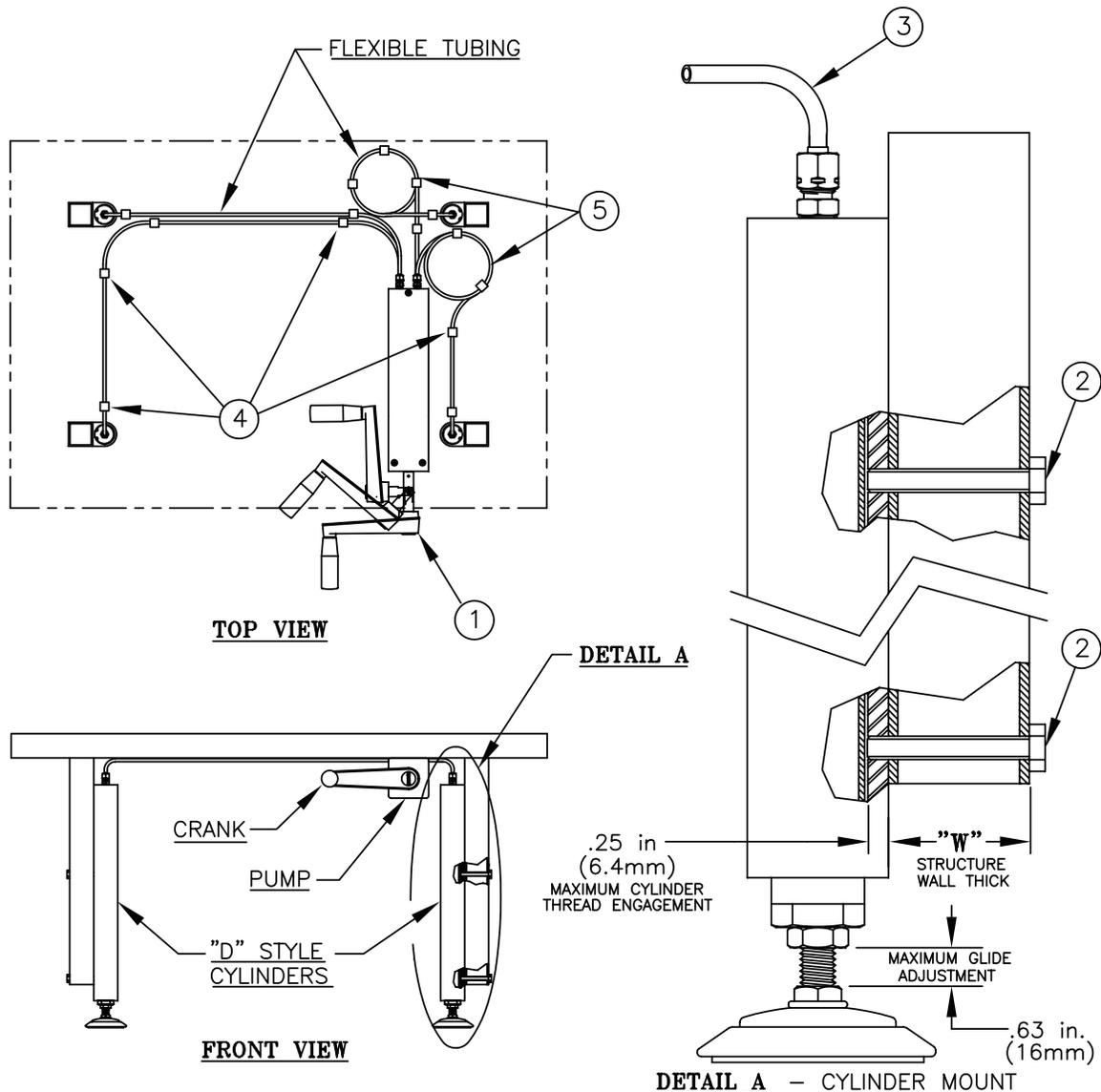
1. Pump should be mounted to structure so that the pump crank is easily accessible by user in its folded position.
